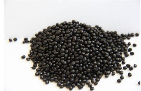
Unlike standard conductive compounds, which have very limited dilution potential, CABELEC CC6135 conductive concentrate can be diluted with a high quantity of natural resin (see graph below). This allows users of CABELEC CC6135 conductive concentrate to benefit from the versatility of this concentrate and from enhanced physical properties due to higher levels of dilution resin.
