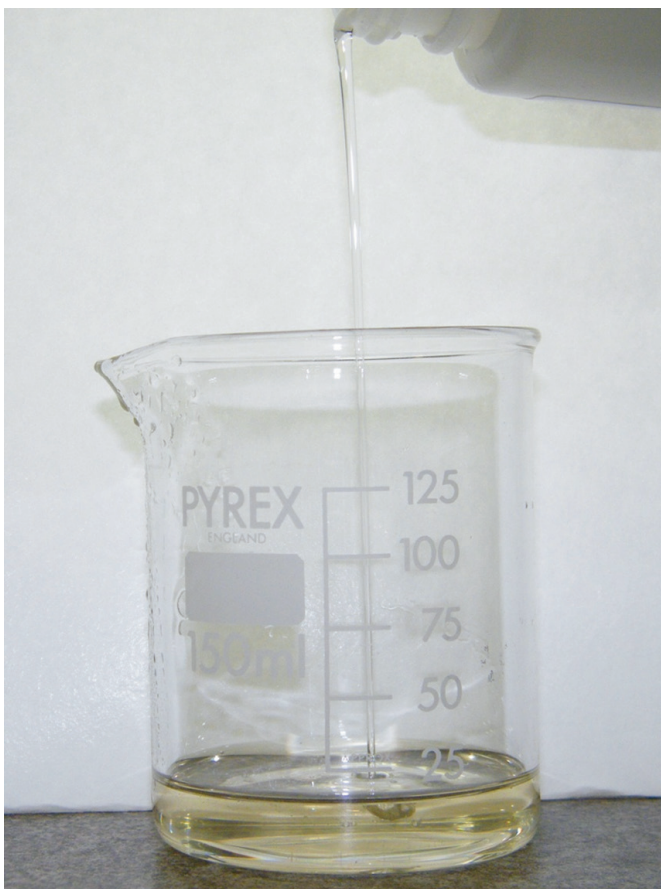
Figure 1. Clear solution of cesium formate in MEG – density 2.22 g/cm 3 .
