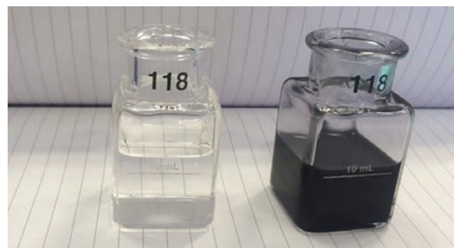
Figure 3. Asphaltenes are removed (left) with PETRODARCO MS activated carbon
