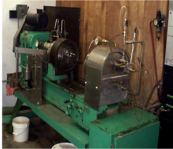
Figure 1 Westport / MI Drilling Fluids' HLT Lubricity Tester.
