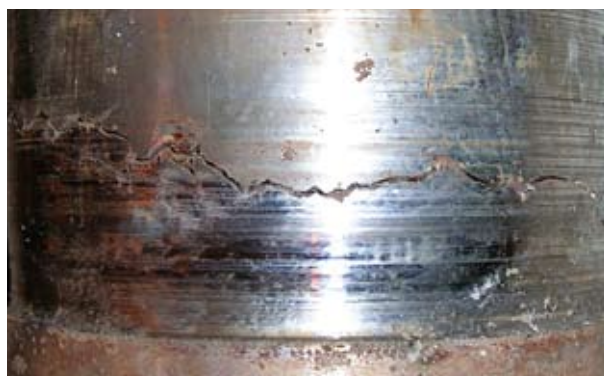
Chloride SCC in CRA
