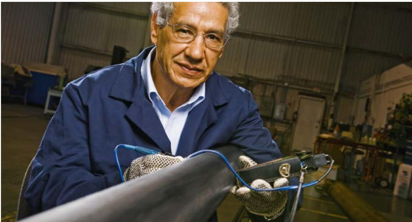
**After six years combating pressures of 14,000 psi and temperatures of 350°F (177°C) the production string was finally pulled from High Island A-5 well #1 situated about 35 miles south of Sabine Pass off the Texas coast. Remarkably, the identification markings on the pipe were still intact.**
